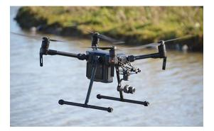
In February, Brian Bailey traveled to Benton County to provide a demonstration of the quadcopter and the process for collection of topographic data. He met with staff from the GIS, Design and Survey Groups to fly their Badger Pit stockpile. Following the flight, he processed the flight data and prepared a ground model which was used to generate a volume of the stockpiles on the site. He discussed specifications of the best equipment to fit their needs in order to implement their own program.
